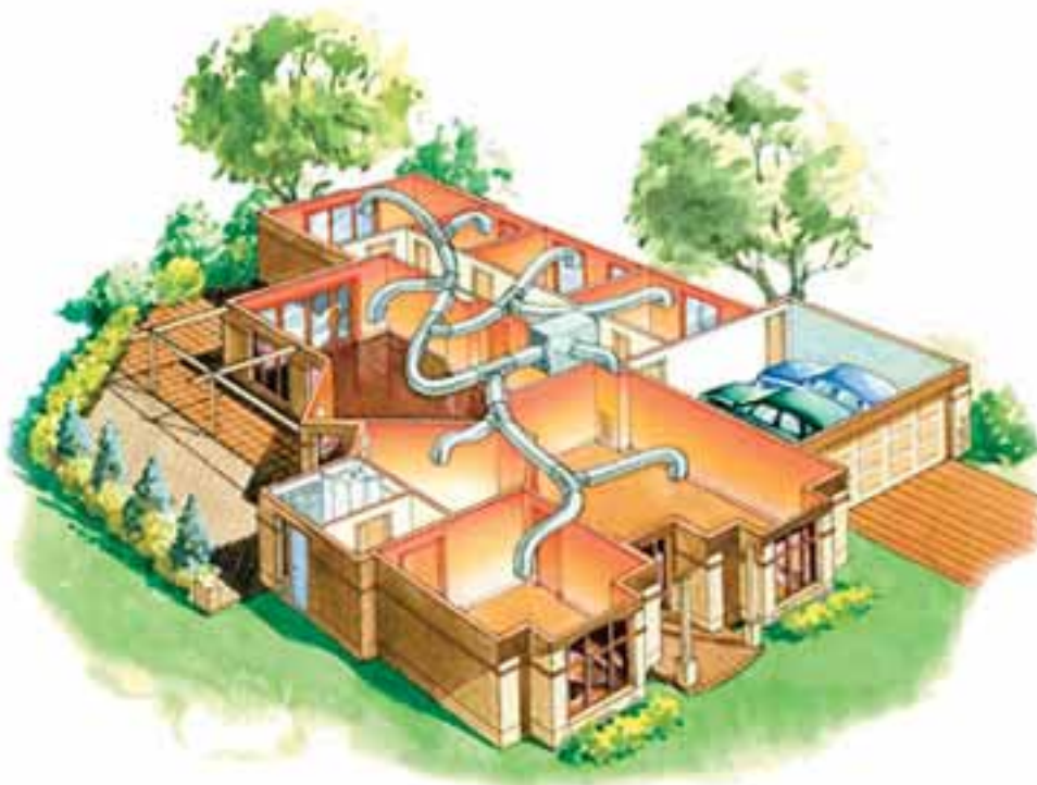
Figure 3: Schematic of Duct Layout for Internal GDH in the Roof Space of a Single Storey Home
