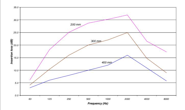
Typical insertion loss (dB) of 3 metre length of perforated duct. Note that the attenuation may be different for different lengths of ducts and data should be used as a guide. The attenuation may be limited by flanking transmission or noise breakout.
